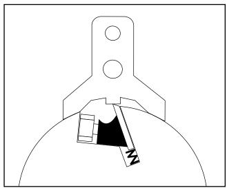
Figure 16. Proper knife setting jig placement.
